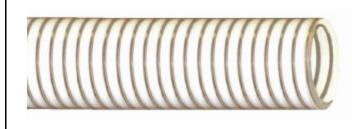
PS1 is a clear, high quality PVC hose for food, dairy, and other sanitary handling, or where see-through flow is required. It complies with 3A Standard No. 20-00 and FDA requirements. Construction includes a white PVC helix.
